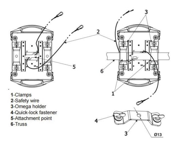
Alternativelly, fixtures handels can be used for safety attachment
