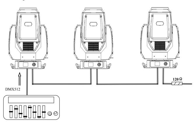
Connect the DMX-output of the first fixture in the DMX-chain with the DMX-input of the next fixture. Always connect one output with the input of the next fixture until all fixtures are connected. **Caution:** At the last fixture, the DMX-cable has to be terminated with a terminator. Solder a 120  $\Omega$  resistor between Signal (–) and Signal (+) into a 3-pin XLR-plug and plug it in the DMX-output of the last fixture.
