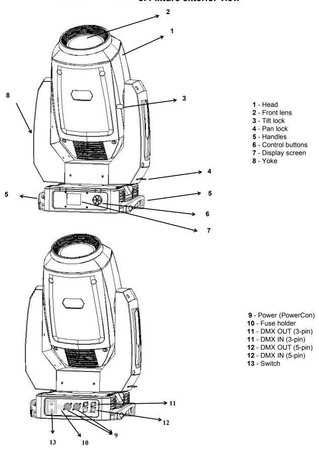
The head has to be locked for transportation- the tilt lock latch (3) and the pan lock latch (4) have to be in the locked positions. To unlock the head, move these latches to unlock positions before operating the fixture.
